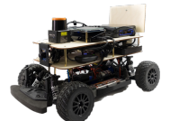
Fig. 5: Prototype 1/10th-scale self-driving car platform.
