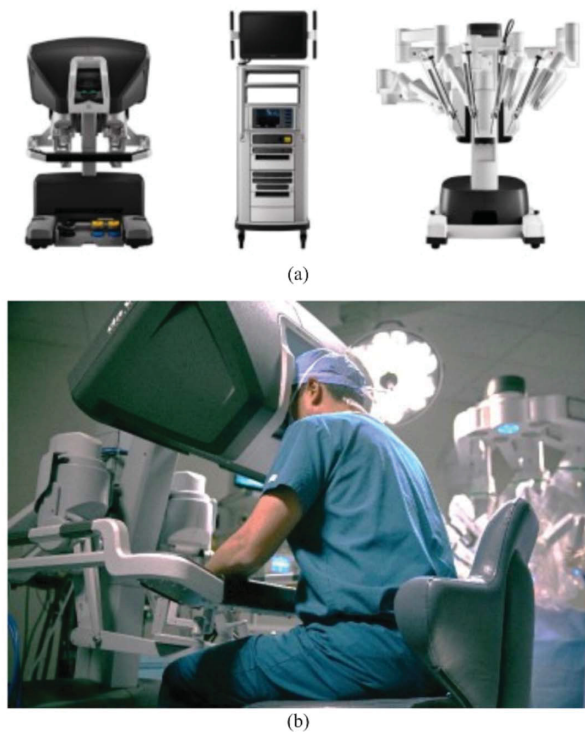
Fig. 1. (a) da Vinci Xi Surgical System. (b) Surgeon's console of the da Vinci Xi System [5]. (© [2022] Intuitive Surgical Operations, Inc.)
