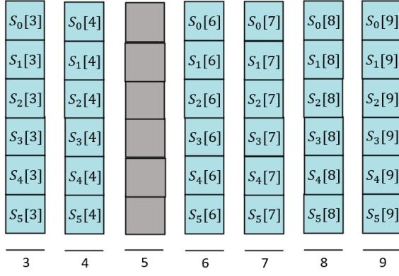
Fig. 8. An example sequence of message packets. Each message packet, S[i] , has 6 total symbols, S_0[i], \dots, S_5[i] , which are contained in the blue boxes. The unlabeled gray boxes are empty and contain no symbols. The numbers under the lines at the bottom indicate the time slots.
