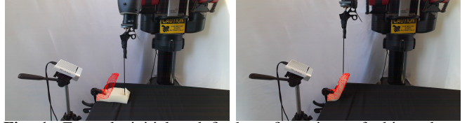
Fig. 1: Example initial and final configurations of object shape control via shape servo with DeformerNet on a physical robot using a laparoscopic tool. We visualize in red the goal point clouds given to the controller.
