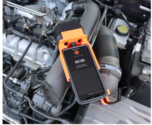
Figure 2: AMP™ device used to record audio for the creation of a vehicle's condition report and subsequently used for the creation of our engine fault dataset.
