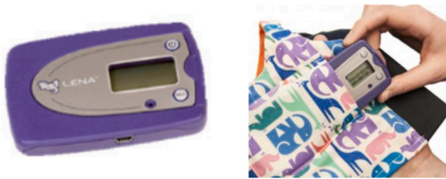
Fig. 2. LENA recording device, which children wear in the front pocket of a specially designed vest.
