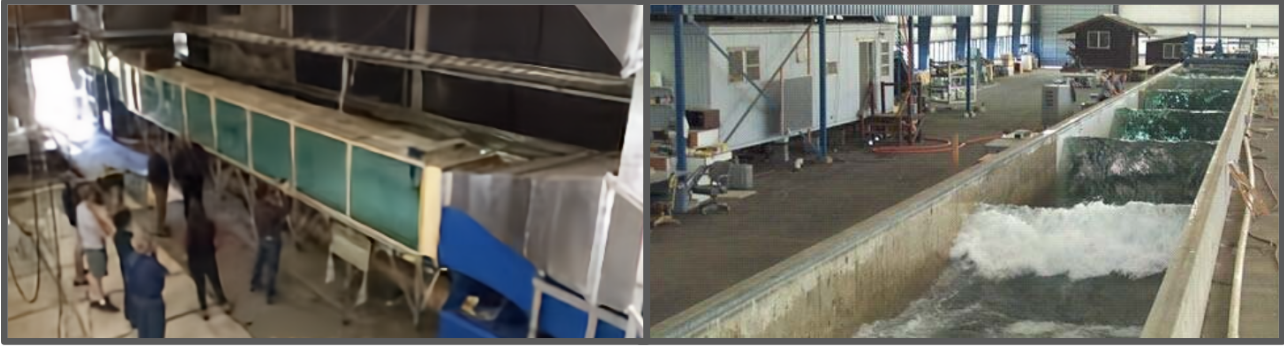
Fig. 1: Wave flume facilities where tsunami-driven debris-field tests were executed. (Left) UW WASIRF. (Right) OSU LWF.
