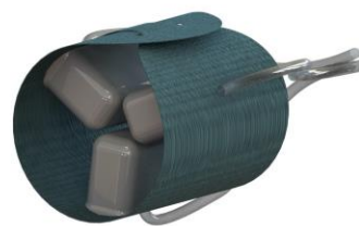
Fig. 1 | Concept and design of the soft robotic aortic sleeve. a , High-fidelity in vivo model of AS based on a biomimetic soft robotic aortic sleeve. The tunability of the sleeve enables the recreation of the haemodynamics of AS and of congenital valve abnormalities, including those of bicommissural and unicommissural aortic valves. b , Two TPU sheets are vacuum formed to a 3D-printed mould. c , The two TPU sheets are heat-sealed together creating three distinct expandable pockets, which are then attached to a strain-limiting fabric through a heat-sealing process that utilizes a negative of the 3D-printed mould. d , Stress-strain response of the TPU and fabric layers under uniaxial tension. Error bars, s.d., n = 3 for each data point. e-f , 3D views of the aortic sleeve with details of the individual TPU pockets, constraining fabric, and hydraulic lines for actuation. g , FE model illustration including a 3D representation of the soft robotic sleeve on the ascending aorta. RV, right ventricle.
