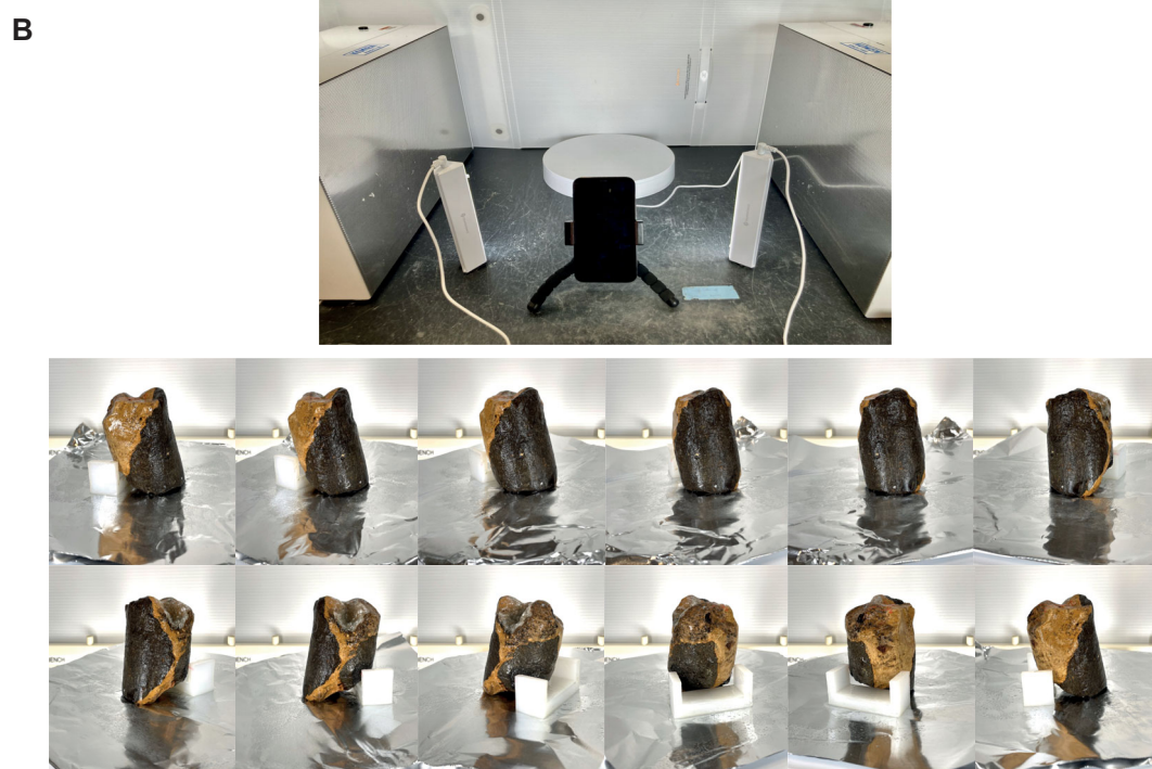
Figure F20. A. DMT CoreScan3 workstation on JOIDES Resolution with example of 3-D high-resolution image created using novel methods developed during Expedition 390. B. Foldio workstation with rotating stage and camera positioned to take multiple time-lapsed images of core pieces as it rotates. These images were taken to preserve information on pieces fragmented for microbiological sampling.
