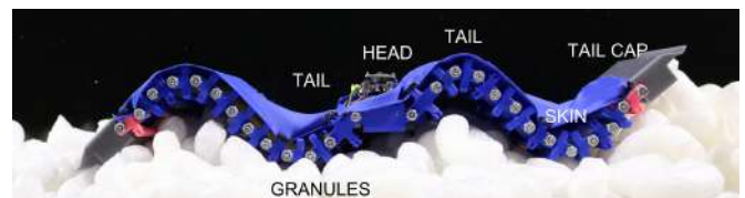
Figure 1. Untethered, double-tailed SAW robot on granules.
