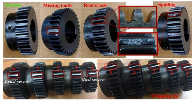
Fig. 4. 9 fault types on pinions, including 5 chipping tip types with 5 different severities.
