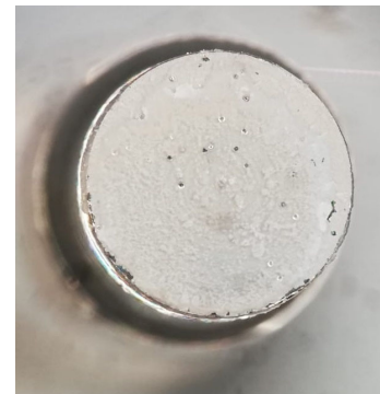
Figure 13: Cohesive failure in adhesive bond
