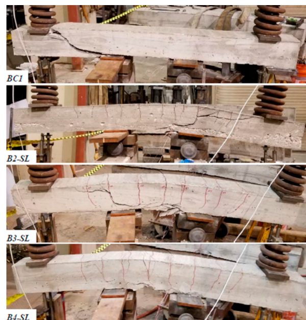
Figure 11. Beam series I failures.
