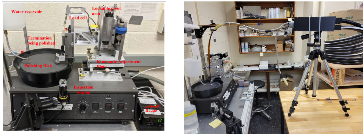
Figure 6. (Left) Custom polisher with inspection microscope which uses two illumination modes to characterize the quality of surface finish. The circumferential illumination mode is especially useful for detecting digs in the surface of a fiber whereas the axial illumination mode seems to be more sensitive to light scratches especially when polishing with very fine lapping paper. (Right) Object array being polished on our custom polisher. The sky array is underneath the tripod awaiting its turn. Any ferrule must be brought to completion before removing it from the polisher in order to prevent faceting.
