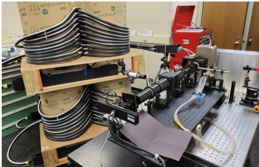
Figure 1. Completed NIR fiber cable set up on TSW. Four sections of conduit, each nearly 40 meters long, are spooled in figure-eights on the left.
