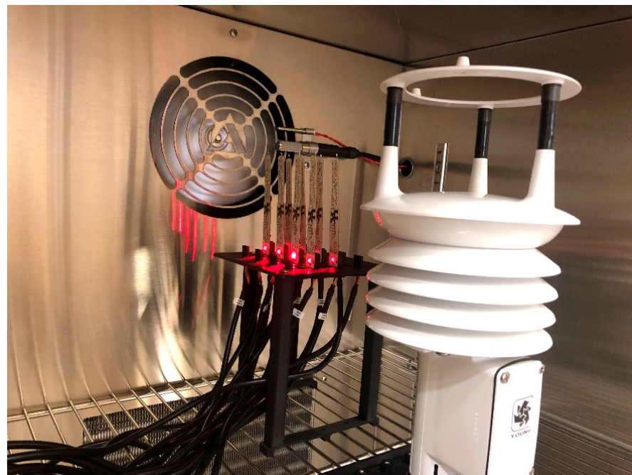
Figure 5. Eight PTH Probes in an environmental chamber. The environmental chamber's temperature and relative humidity sensors and the weather station's barometric pressure sensor were used as reference instruments for calibration and validation. The weather station's ultrasonic anemometer also confirmed that airflow exceeded 1.0 m/s to achieve manufacturer-specified sensor response times.
