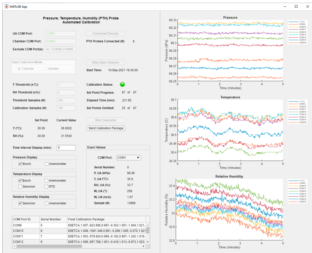
Figure 8. Automated calibration program graphical user interface developed in MATLAB App Designer environment.
