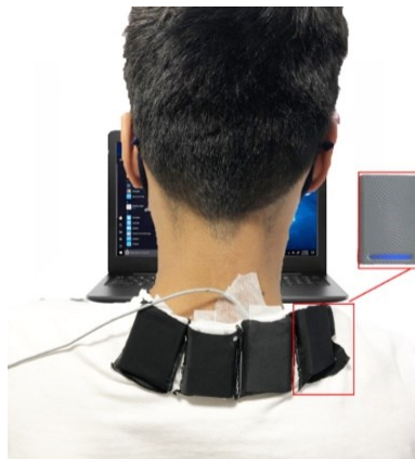
Figure 1: A subject of the local cooling group in a test session with the wearable cooling device. The inner surface of the device was directly contacted with skin by tailoring the T-shirt. The cable was connected to a fast-responsive skin temperature sensor.
