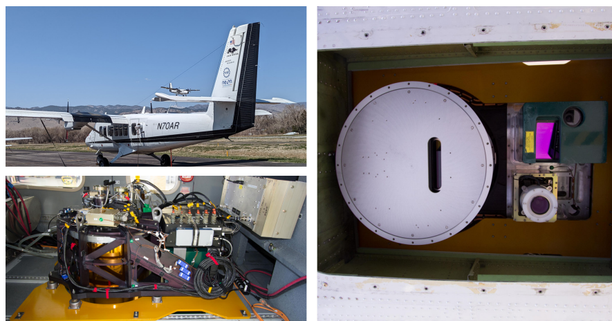
FIGURE 1 Top left—Twin Otter aircraft preparing for calibration flights; bottom left—Airborne Observation Platform payload installed in aircraft (instrument racks not shown); right—spectrometer, lidar and camera sensors viewed from below
