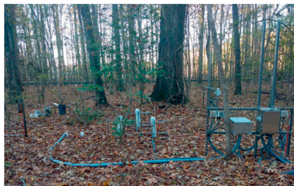
FIG. 5. The NEON soil plot design. (left) Conceptual design and location of individual instruments. For a full description of all sensors, please see Table 5 [in short, heat flux plate (S01), temperature profile (S02), moisture profile (S03), CO 2 profile (S04), throughfall precipitation collector (S05), upward-facing quantum-line photosynthetically active radiation sensor (S06), net radiometer and infrared biological temperature (S07), and relative humidity sensor (not shown)]. (right) Example of an actual soil plot at the NEON Lenoir Landing (LENO) site.
