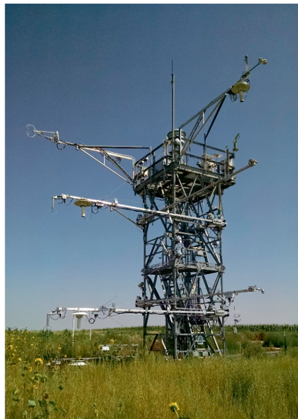
FIG. 4. The NEON tower design. (left) Conceptual design and location of individual instrument assemblies for a four-level tower. For a full description of all sensors, please see Tables 1–4 [in short, 2D sonic anemometer (T01, T03, T05), shielded and aspirated air temperature sensors (T02, T04, T06, T07), eddy covariance boom (T08; including 3D sonic anemometer, infrared gas analyzer and attitude and motion reference sensor), environmental enclosure (T09), secondary precipitation gauge (T10), spectral photometer (T11), radiation boom (T12), pyranometer (T13), sunshine pyranometer (T14), net radiometer (T15), up-facing and down-facing photosynthetically active radiation sensors (T16), and midlevel radiation boom (T17, T18, T19; including an up-facing photosynthetically active radiation sensor and an infrared temperature sensor)]. (right) Example of an actual four-level tower at the NEON Sterling (STER) site.
