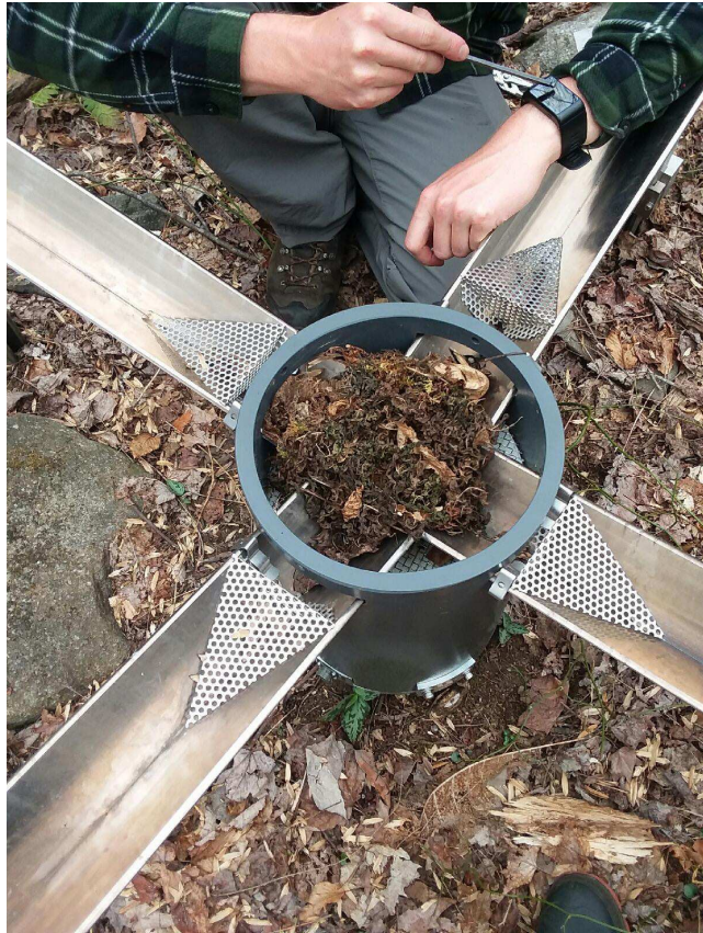
FIGURE 6 An animal nest discovered in a throughfall precipitation gauge at the NEON Great Smoky Mountains National Park (GRSM) site, causing diminished rainfall measurements. A data quality trouble ticket was created and reviewed via the issue management system. Affected data were manually flagged.
