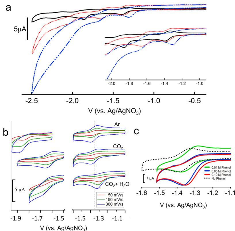
**Figure 1.** CV measurements of 0.10 mM solution of **1** in dry THF. (a) CV under argon (black solid curve), CO<sub>2</sub> (red dotted curve), and CO<sub>2</sub> and water (5% v/v, blue dashed curve). The inset is the zoom-in of the selected voltage range. (b) CV scans at various scan rates under the three reaction conditions. (c) CV scans with various amounts of phenol added under an argon atmosphere.
