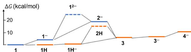
**Figure 3.** Comparison between the calculated energetics of the proton-coupled (orange lines) and unprotonated (blue lines) pathways for  $\text{CO}_2$  activation at the equilibrium potential to produce  $1H$  ( $-1.33\text{ V}$ ).
