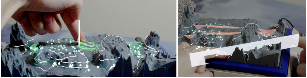
Fig. 5. Streamlines are interactively seeded by moving a finger around on the surface of the physicalization and releasing (left), while cutting planes are created by using two fingers (right).
