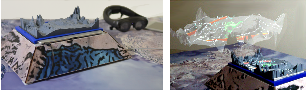
Fig. 4. (Left image) The physicalization and force-sensing surface are placed on a truncated pyramidal base. The base is situated onto a large fabric poster with contextual NASA satellite imagery around the Filchner-Ronne ice shelf in the Antarctic. The imagery is not to scale with the physicalization. (Right image) Worlds-in-miniature allow the user to view their data at multiple scales. All interactions still take place on the physicalization; when users are focused on the larger world, the physicalization acts as a haptic proxy.
