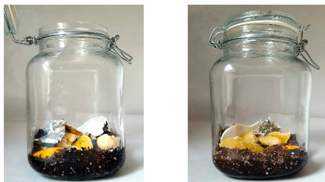
Figure 1. Physical model of landfill bottles in open and closed systems.
