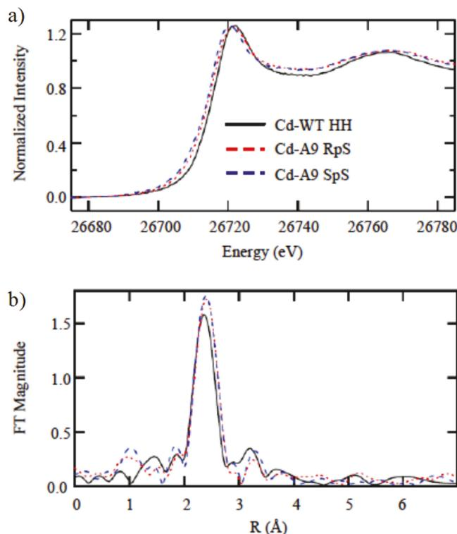
Fig. 7. Cd K-edge and EXAFS Fourier transforms (over the range of  $k = 2\text{--}11 \text{ \AA}^{-1}$ ) for wild type, A9- $\text{S}_{\text{Sp}}$  and A9- $\text{S}_{\text{Rp}}$  tHHRz. a) The Cd X-ray absorption edge is slightly lower for the tHHRz A9-S samples (dashed). b) Longer distance and higher amplitude for first-shell scatterers in both of the tHHRz A9-S samples (dashed) in comparison with WT (solid).
