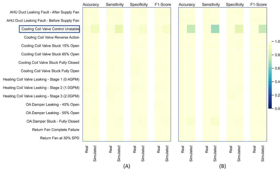
Fig. 2. Performances comparisons between random forest (Fig. 2A) and SVM (Fig. 2B) with 80% training size and 10-fold CV. “Real” means real building data and “Simulated” means simulated building data.
