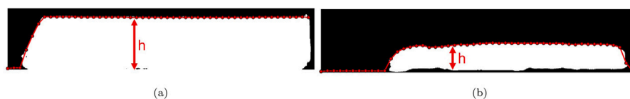
Fig. 4. An example of the masks of the regressing fuel with the profile height tracking. (For interpretation of the references to color in this figure legend, the reader is referred to the web version of this article.)
