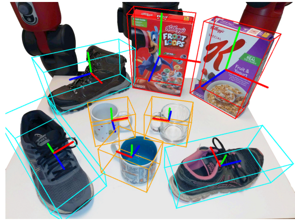
Fig. 1. Given a single RGB image containing previously unseen instances of known categories (in this case cereal boxes , cups , and shoes ), our proposed method detects objects and estimates 6-DoF poses and 3D bounding box dimensions up to a scale factor. We use a separate network for each category.
