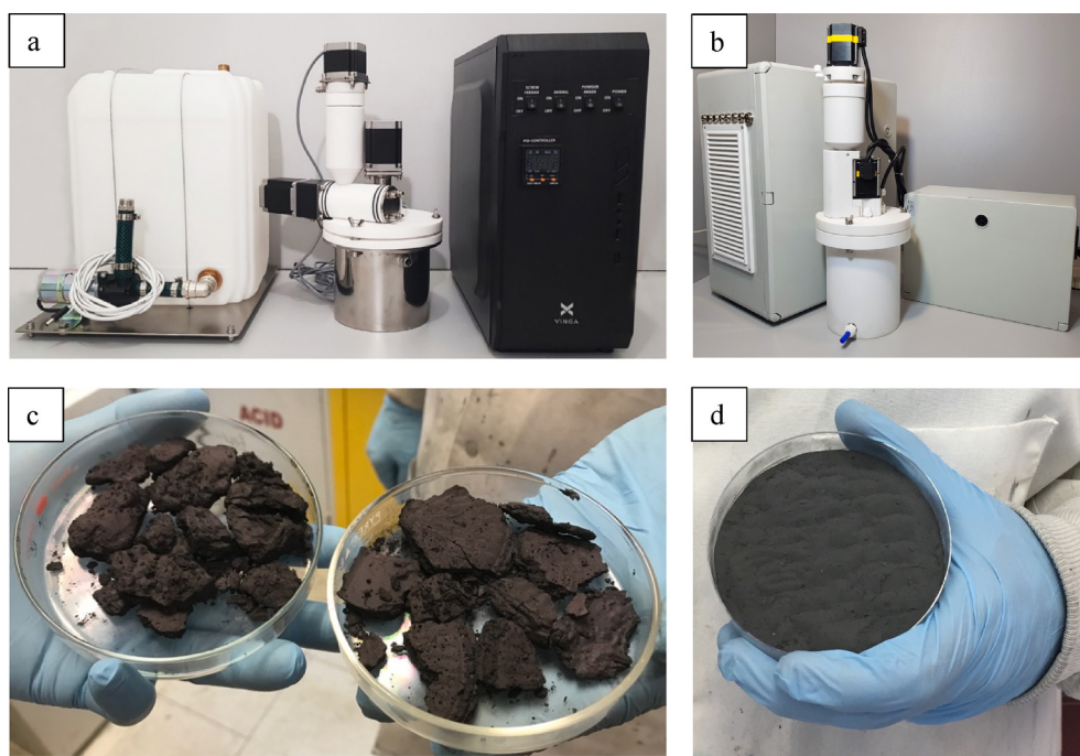
Fig. 2. Commercial laboratory scale reactors designed for synthesis of MXene and dried MXene powders after synthesis. (a) MXR204MCW-0.5L reactor (1L and 2L modifications are available at Drexel University); (b) MXR310-1L reactor with an active cooling and heating system and the all-Teflon body; (c) about 70 g of multilayer Ti_3C_2T_x and (d) about 40 g of Mo_2TiC_2T_x . (a, b) – courtesy of Materials Research Center, Ukraine. Ti_3C_2T_x was synthesized by M. Alhabe and Mo_2TiC_2T_x was made by P. Lelyukh.
