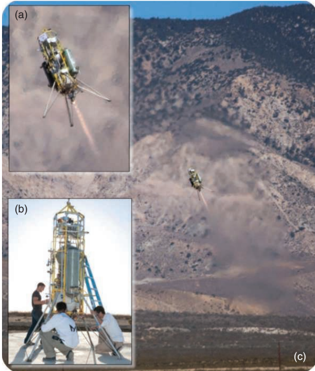
FIGURE 19 The Masten Xombie rocket near the end of a 750-m divert maneuver. (Source: [37, Fig. 1]; used with permission.) (a) Close-up of the rocket executing an optimal divert trajectory. (b) Preflight checkout by the Masten Space Systems staff. (c) A zoomed-out view with the Mojave desert in the background.
