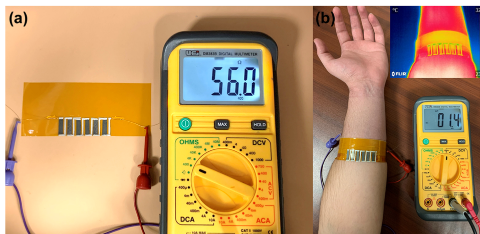
Fig. 6 Performance of a wearable TEG. (a) Internal resistance of the TEG fabricated using six silver–selenide films. (b) Digital photograph of 1.4 mV open-circuit voltage generated at a \Delta T of \sim 1.8 K between the hot side and the cold side of the device. The inset is the corresponding infrared thermal image.
