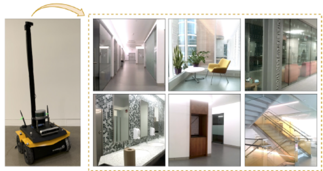
Fig. 1: Photos Captured By AutoPhoto. Left: The AutoPhoto system deployed on Clearpath Jackal robot. Right: Photos autonomously captured by AutoPhoto. See Fig. 4 for comparisons against initial environment views.
