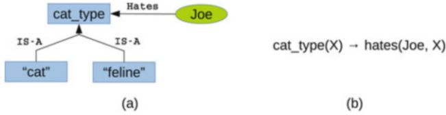
Fig. 3.4 Modeling morphological variation, (a) entity-relationship diagram, (b) predicate calculus
