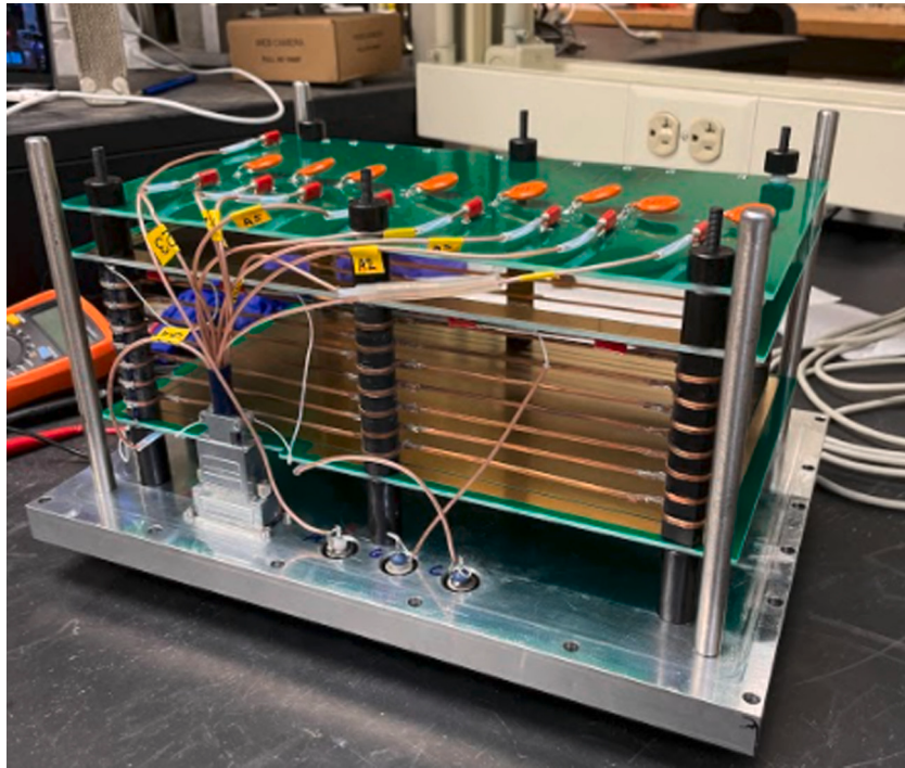
Fig. 3. The top plate of the MONICA detector inverted on a tabletop, with the internal fixtures attached. The green plates are the cathode, Frisch grid, and anode from bottom to top and field cage electrodes surrounding the sides. (For interpretation of the references to color in this figure legend, the reader is referred to the web version of this article.)
