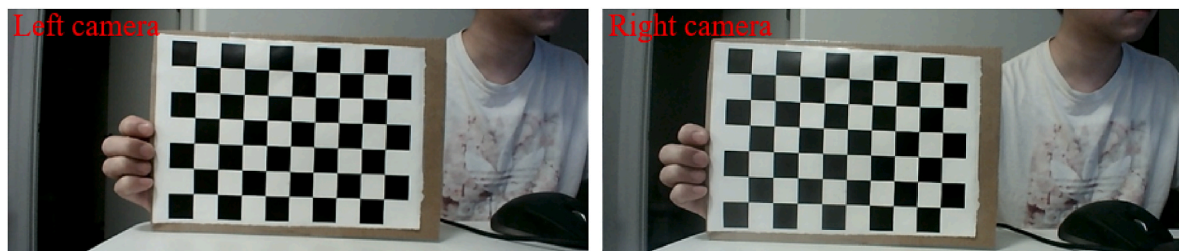
Fig. 3. Calibration of binocular camera using a checkboard with black and white squares. “Left camera” and “right camera” refer to the left and the right telescopes of the binocular camera.
