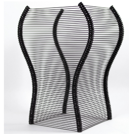
Figure 1: Our system, p5. fab, controls digital fabrication machines from the creative coding environment p5.js. We programmatically generate toolpaths using our library (left) which we can visualize in our user interface with a render command (center). We stream these commands to a desktop FFF 3D printer for fabrication; a photo of the resulting print is shown (right).
