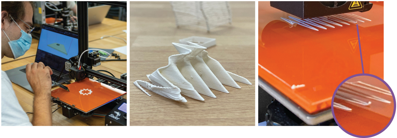
Figure 9: Process pictures from the artist workshop evaluation. Artists leveraged their creative coding skills to quickly begin printing (left). While printing a sinusoidal sculpture (center), A3 struggled with bed adhesion (right). To get the peaks and troughs to adhere, they negotiated their design geometry (wave period) with machine parameters (print speed).
