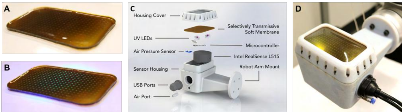
Fig. 2. A. Soft membrane in ambient room light. B. Soft membrane with UV-phosphorescent dot grid pattern activated by 365nm UV light. C. Overview of sensor system. D. Sensor mounted on UR10 robot arm.
