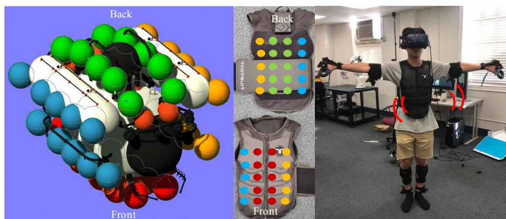
Figure 4. User setup - sphere shaped triggers matching haptic suit feedback points.
