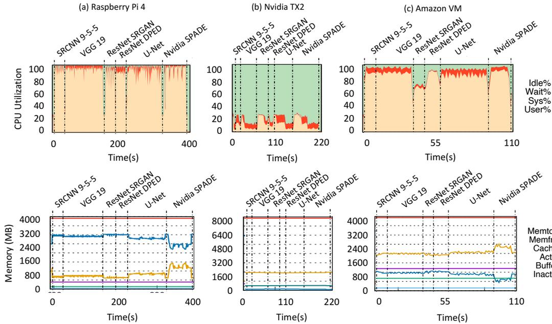
Fig. 4: CPU and memory utilization of image-to-image applications.
