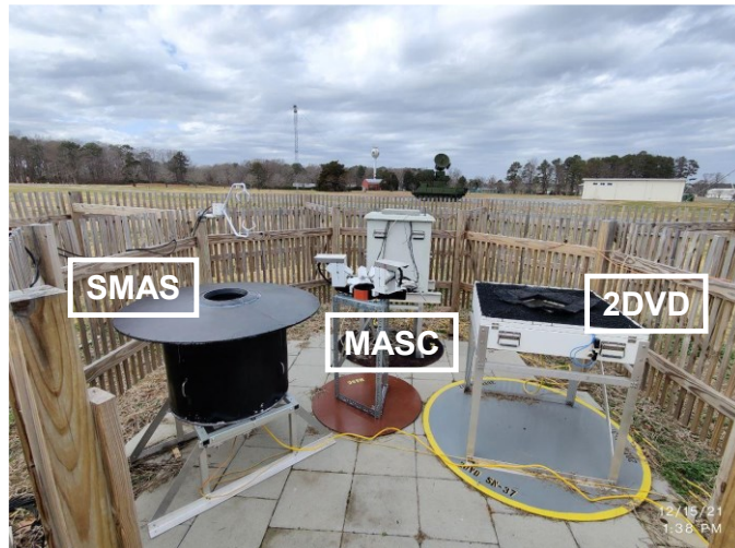
Figure 1. Colorado State University's SMAS and MASC installed within a double-fence windshield at the NASA Precipitation Research Facility, Wallops Island, VA (where PIP and 2DVD are already operational), December 2021.
