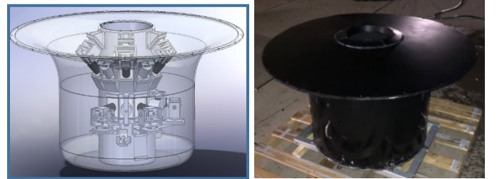
Figure 2. (left panel) CAD model (transparent CAD solid model) of SMAS outer chassis – in Nipher shield shape, which maximally reduces turbulence. (right panel) SMAS prototype outer chassis photograph.
