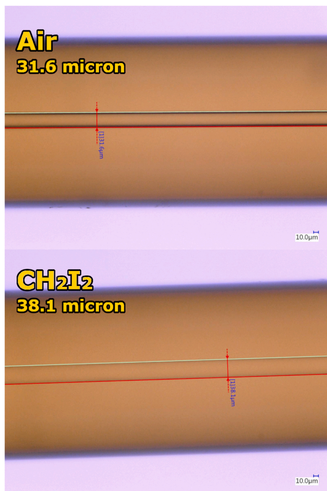
Fig. 5. Effect of fluid refractive index on the optically perceived diameter in transverse imaging. The manufacturer stated and cross section measurement optical diameter was 25.2 \pm 0.2 \mu\text{m} .
