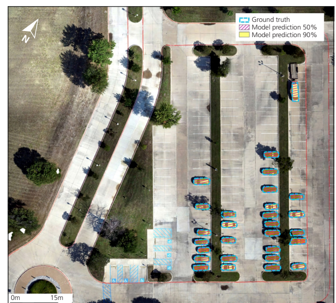
Figure 11. Neural-network-based prediction of cars at 50% and 90% confidence scores
