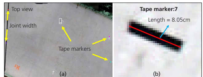
Figure 5. Bridge deck inspection: (a) locations of a few markers, (b) pixel view of tape marker 7 on scaled image from UAV-CRP technology
