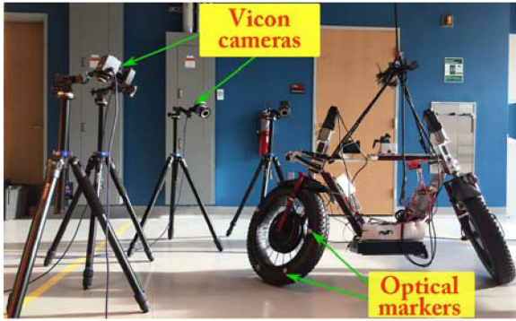
Fig. 5. Experimental setup for validation of the steering mechanism and balance torque model.
