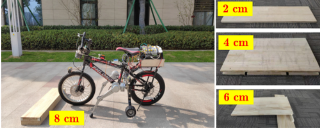
Fig. 5. Bikebot experiments for various obstacle crossing tests. Wooden blocks with different heights are used as obstacles in experiments.
