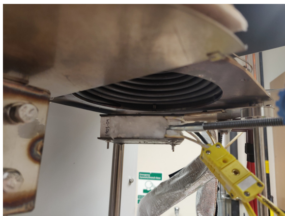
Fig. 2 DFT being tested using an ASTM E1354 cone calorimeter heating element
