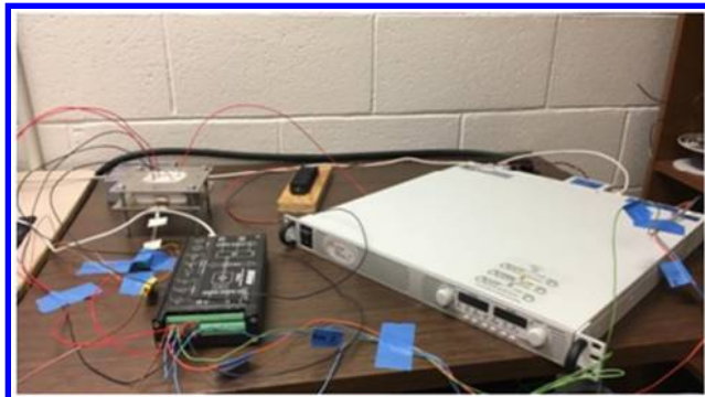
Fig. 10 Test cell, bus bar, DAQ, and dc power supply.
