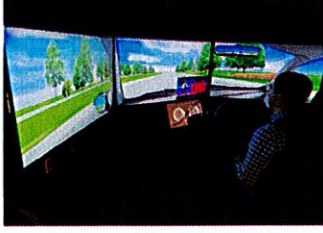
Fig. 2. Experiment setup—the video (non-driving-related task) was located in the bottom corner of the main screen.
