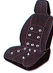
Fig. 3. Distribution of tactors in the seat back and seat pan.
