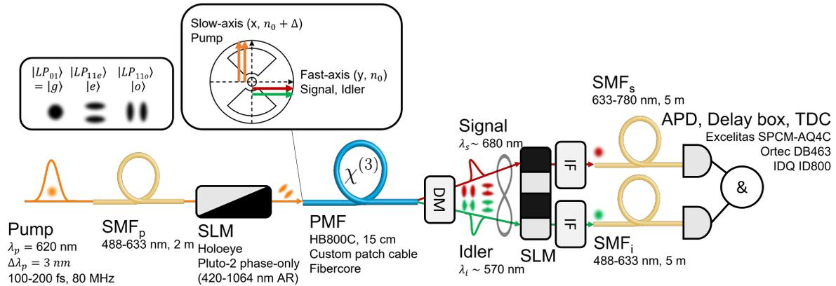
Fig. 1. Simplified experimental setup. SMF: single-mode optical fiber, SLM: spatial light modulator, PMF: polarization-maintaining optical fiber, DM: dichroic mirror, IF: interference spectral filter, APD: avalanche photodiode, TDC: time-to-digital converter. Polarization optics are omitted for simplicity.
