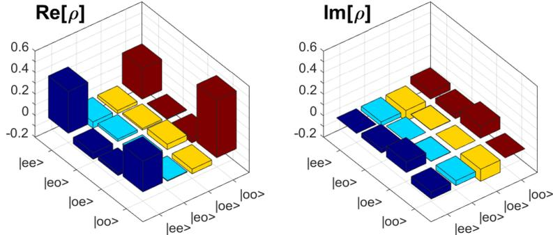
Fig. 2. Real (left) and imaginary (right) parts of the experimentally reconstructed density matrix  $\rho$  of a transverse-mode entangled state via quantum state tomography, with axes labeled with the signal and idler transverse mode states,  $|T_s T_i\rangle$ .
