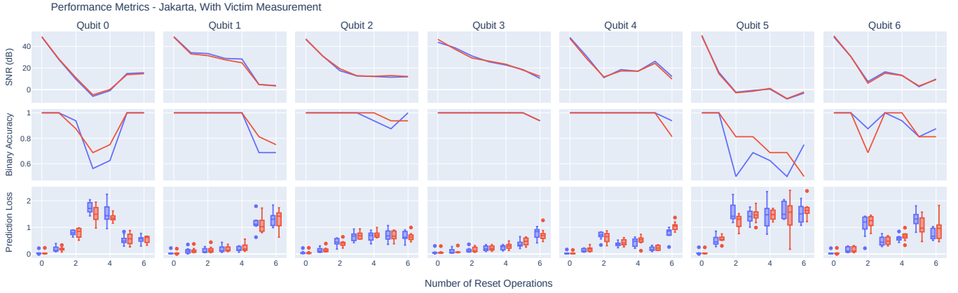
Figure 5: Training (blue) and testing (red) fidelity under various metrics on each qubit of Jakarta with victim measurement, with respect to the number of reset operations between the victim and the attacker. For the angle prediction loss, the error bars represent variations over \theta .
