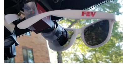
(b) The camera of the vehicle is fitted with sunglasses to reduce bright reflection and unwanted glare.
