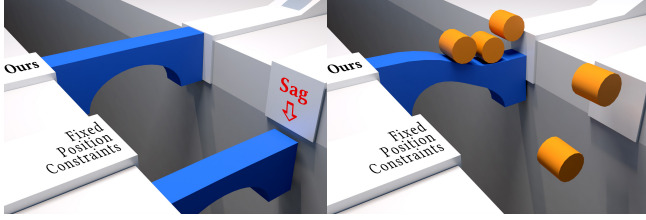
Fig. 5. A soft bridge using our initialization and fixed position constraints. In the latter case, contacts are treated as static and friction is not handled. Our initialization is able to correctly solve for friction and wedge itself between the two cliffs and (left) maintain the initial state until (right) the barrels overwhelm the bridge’s friction. Initializing using fixed position constraints, on the other hand, causes the soft bridge to slide down as soon as the simulation begins.
